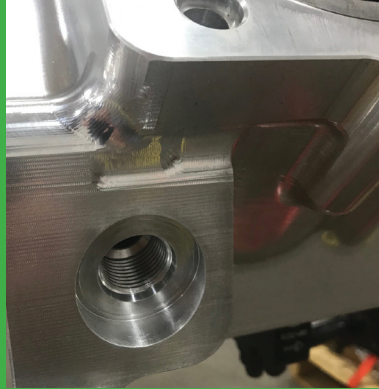
Lifter Valley/Cam Tunnel Scavenger Drain Fitting.
